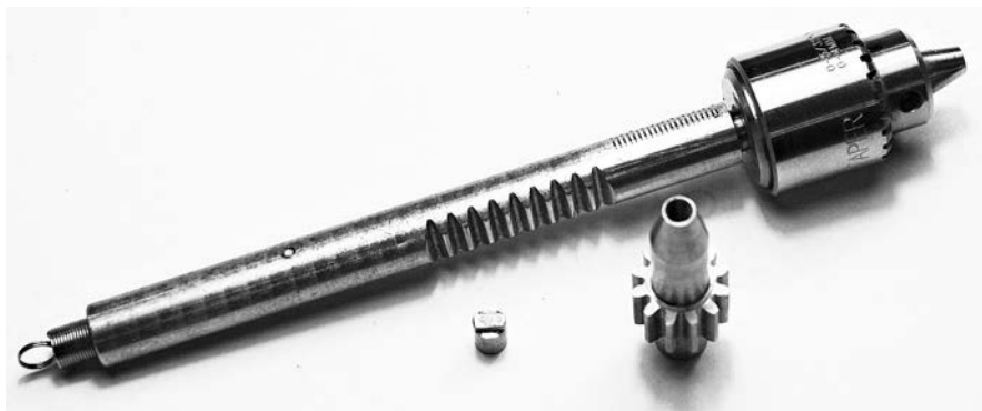
Figure 6 The completed quill, pinion spindle and key
